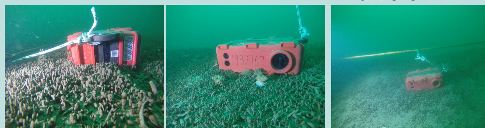
Seabed receivers : 4C GPR Nodes from Sercel
